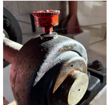
Fig. : A lubricated plain bearing casing from the triple refractor of the Neuchâtel Observatory.
