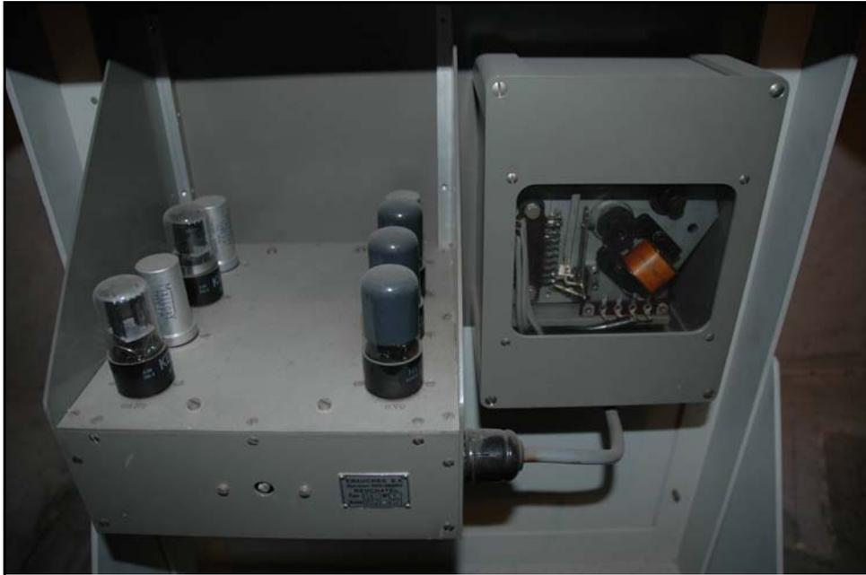
Image 9.15 : Compartiment 5, horloge Oscilloquartz
