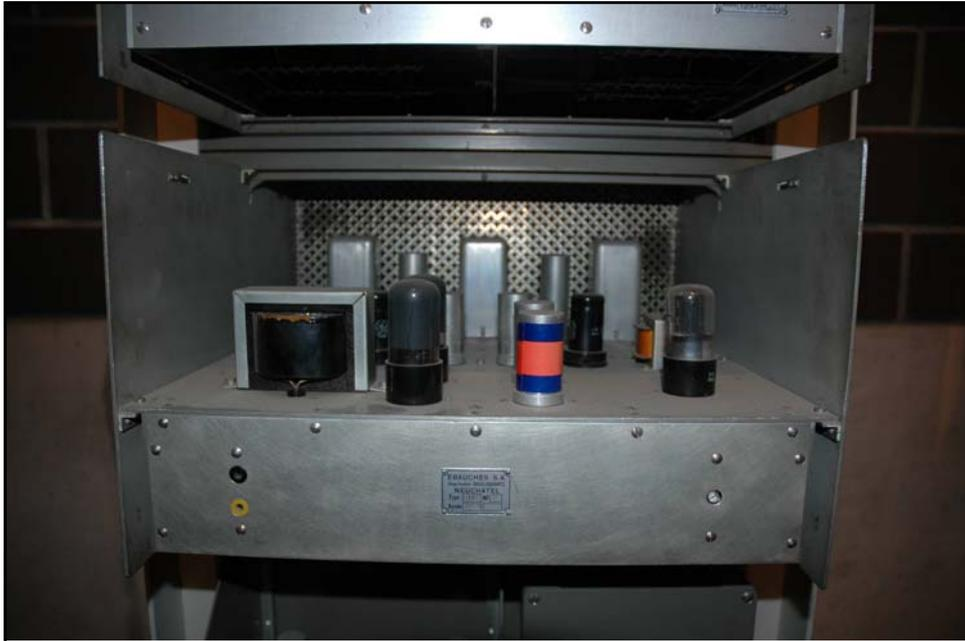
Image 9.13 : Compartiment 4, horloge Oscilloquartz
