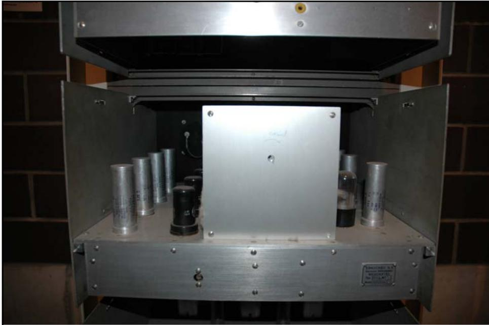
Image 9.11 : Compartiment 3, horloge Oscilloquartz
