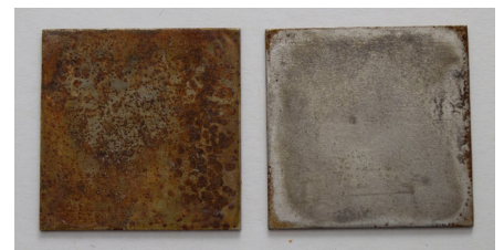
Fig. : steel plates artificially corroded : on the left untreated, on the right treated with bacterial metabolites.
