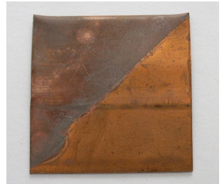
Fig. : naturally corroded copper plate : top-left half untreated, bottom-right half treated with fungi.
