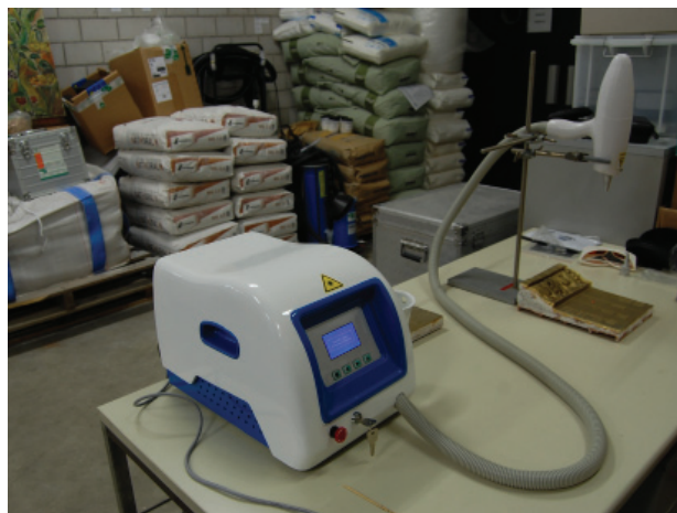
Fig. 2: Laser cleaning tests on a test panel.
