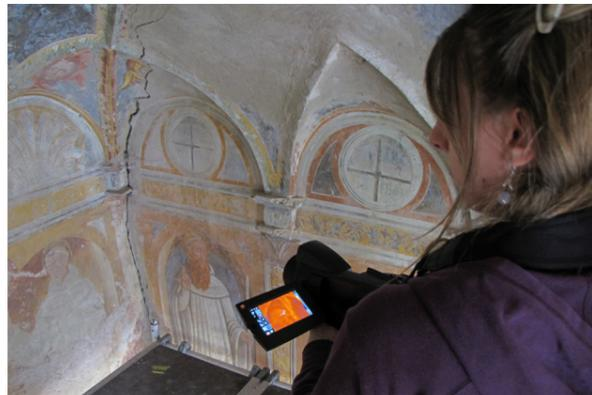
Fig. 2: Investigations using passive thermography to detect delamination of plaster, San Nazario Church, Sonvico - Dino, exterior chapel, west wall. SUPSI - PoliMi. May 2013
