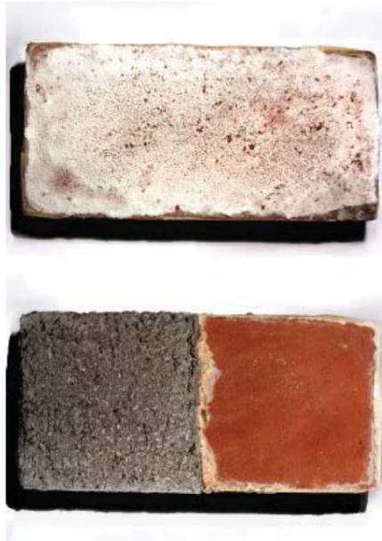
Fig. 2: Upper picture: Painted plaster samples contaminated by hygroscopic salts after the contamination. Lower picture: Painted plaster samples at the conclusion of the 90 days of application of sacrificial plasters: on the left the sacrificial plaster, on the right the original painted surface of the sample without salt crystallization.
