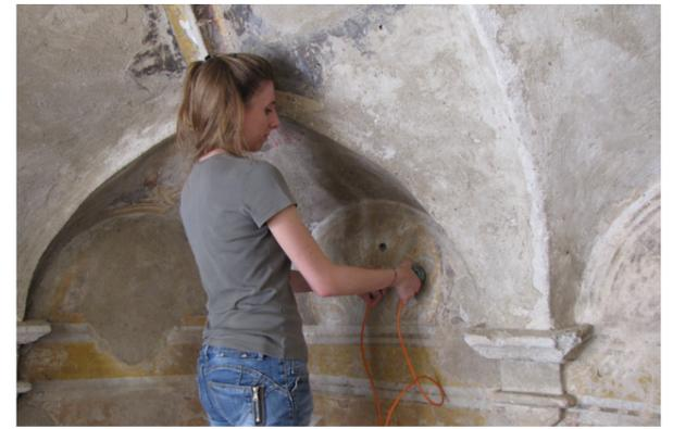
Fig. 3: Test with ultrasonic instrumentation for the evaluation of detachments, San Nazario Church, Sonvico - Dino, exterior chapel, west wall. SUPSI - Boviar. July 2013
