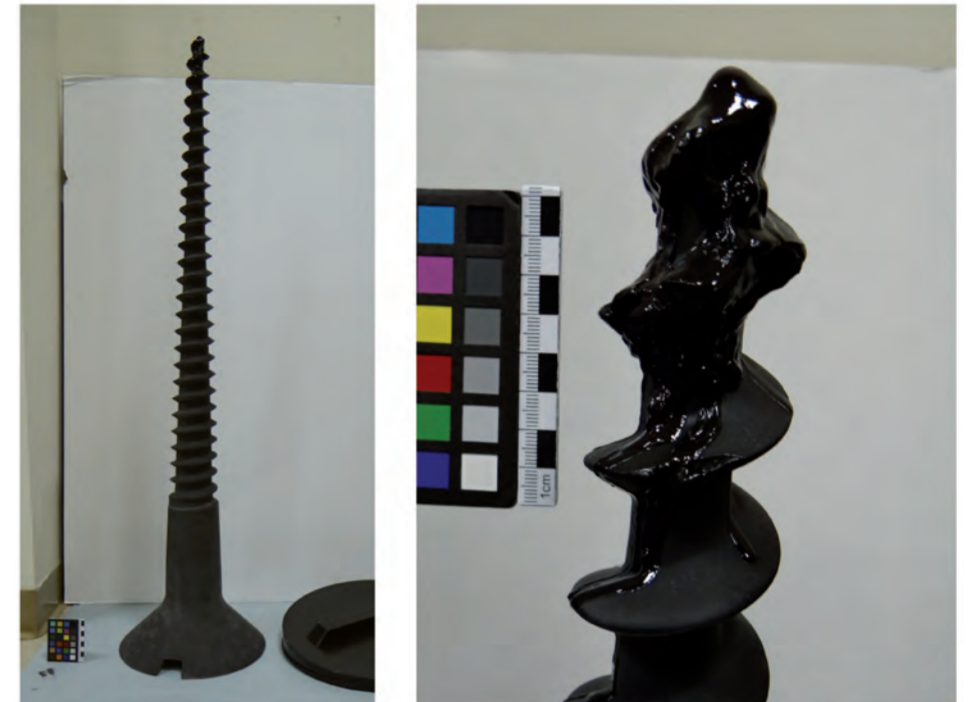
Fig. 3: Sculpture exhibiting material softening only, through the formation of viscous material that results in the loss of form.
