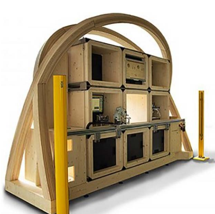
The prototype microfactory is made from Swiss wood: a renewable material that absorbs vibrations.
